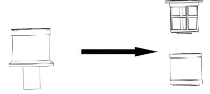
4. Clean the mesh filter and air intake filter by washing them thoroughly.
