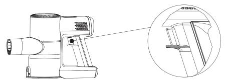
Press the MAX button to switch between Regular mode, which is ideal for daily cleaning, and Max mode, perfect for deep cleaning tasks like carpet
