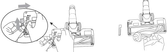
2. Use scissors to remove any hair and debris wrapped around the roller.
