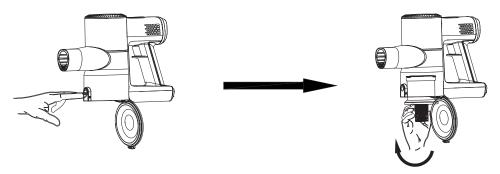
**3.** Remove the HEPA filter, then lift up the cover to access the internal components.
