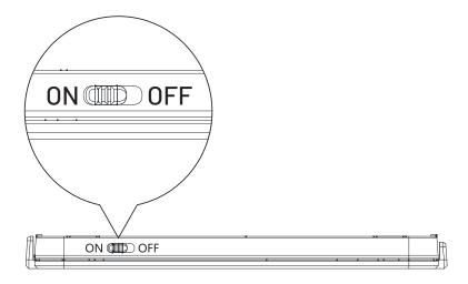
1. Slide the keyboard's on/off switch to the "on" position, and select the Bluetooth mode when the red light is visible. Then press Fn+C to start pairing when the blue light begins flashing.
