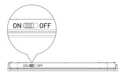
1. Slide the keyboard's on/off switch to the "on" position, and select the Bluetooth mode when the red light is visible. Then press Fn+C to initiate pairing when the blue light begins flashing.
