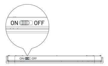
1. Slide the keyboard's power switch to the "on" position. Select the Bluetooth mode when the red light is visible. Then, press the Fn+C keys to initiate pairing when the blue light begins flashing.
