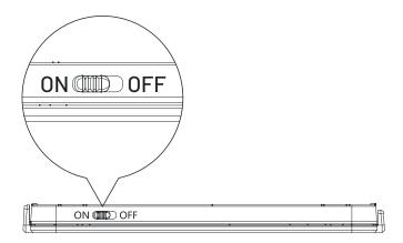
1. Slide the keyboard's on/off switch to the "on" position and select the Bluetooth mode when the red light is visible. Then, press Fn+C to begin pairing when the blue light starts flashing.
